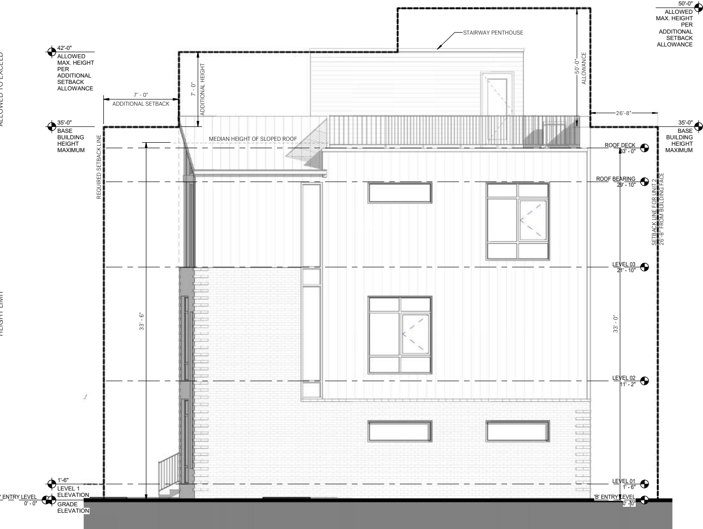
UNITS 3-5 - SOUTH ELEVATION
