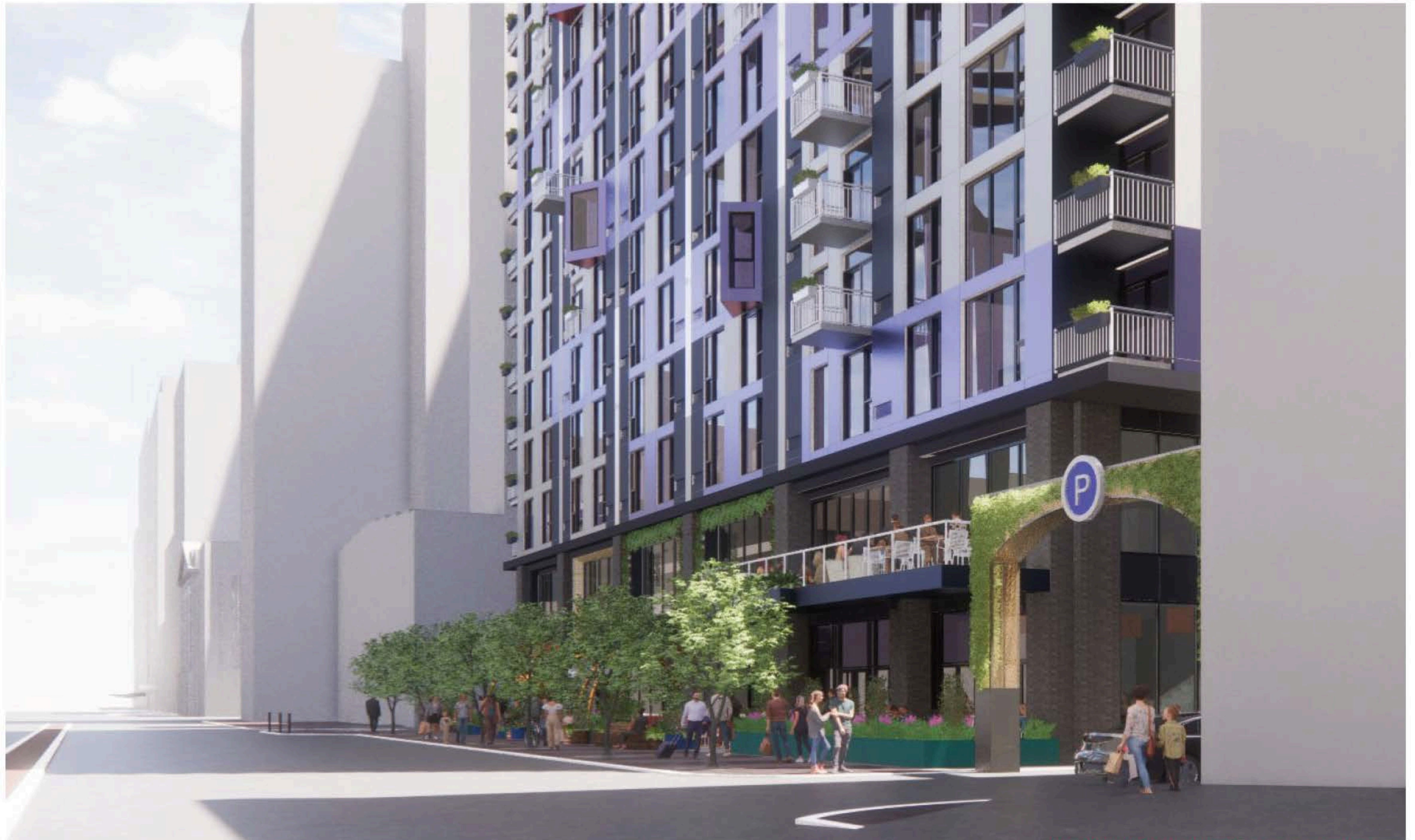
EAST BOUND OPTION 1 - Portal flush with building facade Island recessed further back for car queue line.
