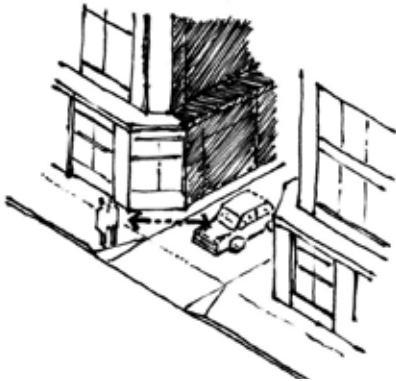
Parking access behind buildings; chamfered corners increase visibility and safety
