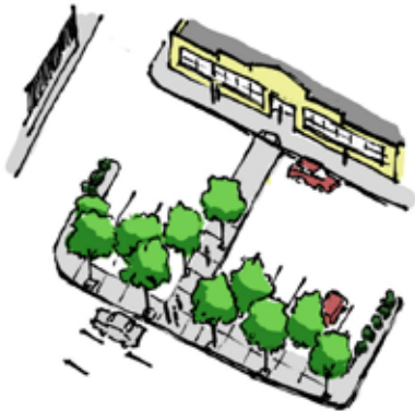
Pedestrian connector from parking to the front of the building
